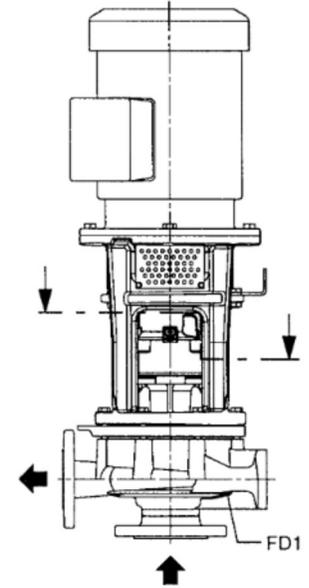
**Connections for horizontal and vertical installation**
