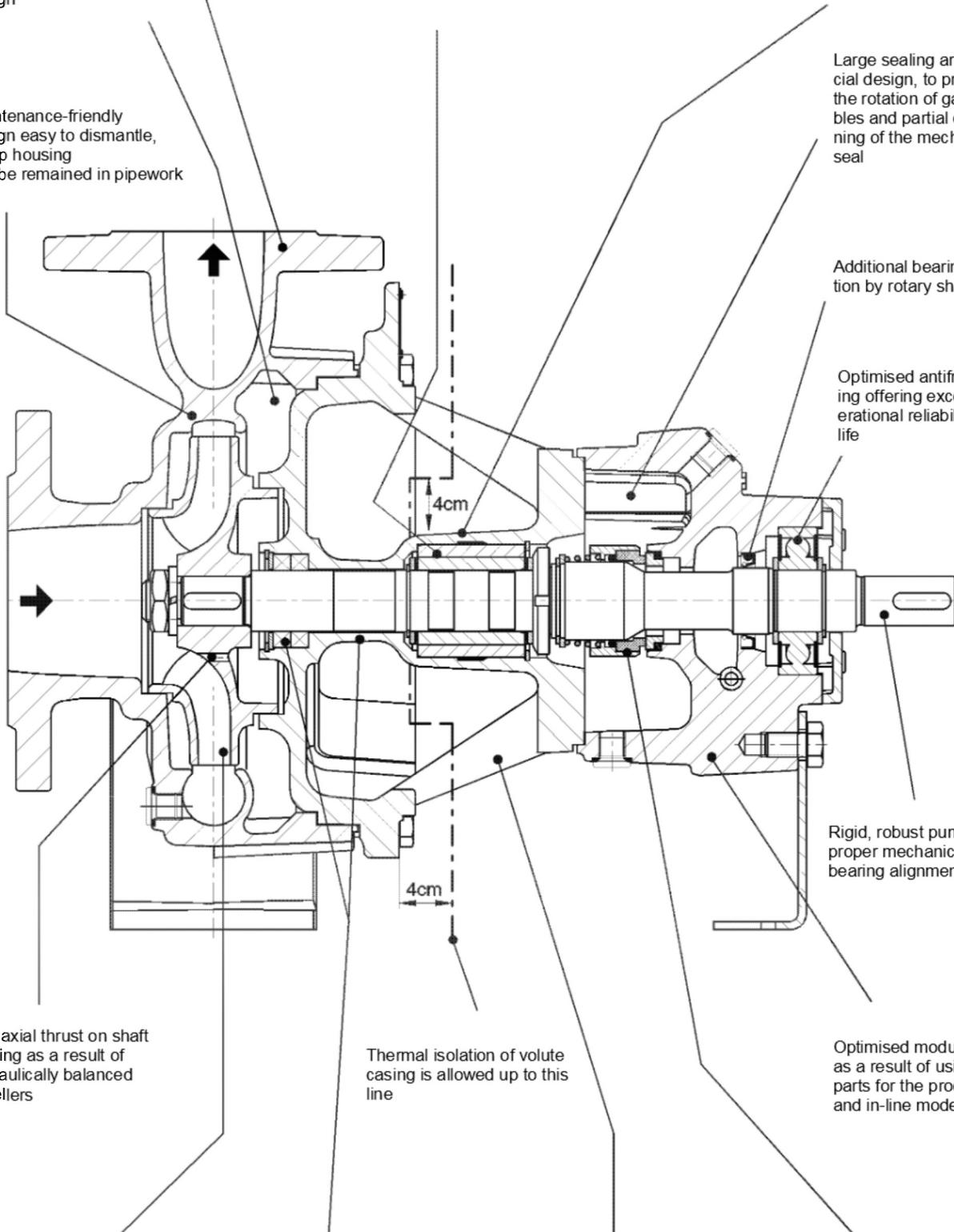
**Interchangeability of components on bearing bracket sizes 1 and 2**
