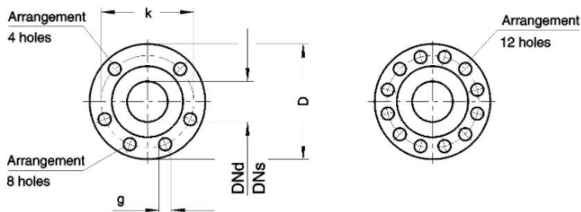
Arrangement of connections – Series NTWH
